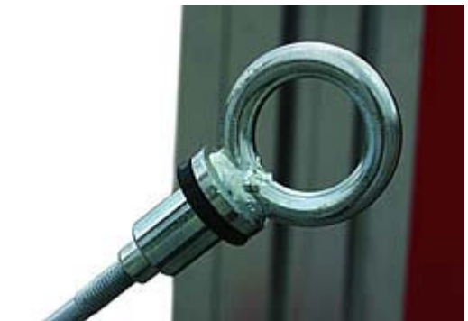
7. Fit the lifting eyes to secure the unit
