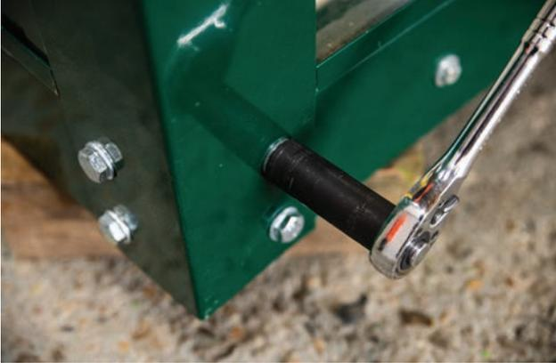
8. Repeat the fitting of panels and outer corner posts for the three other sides.
