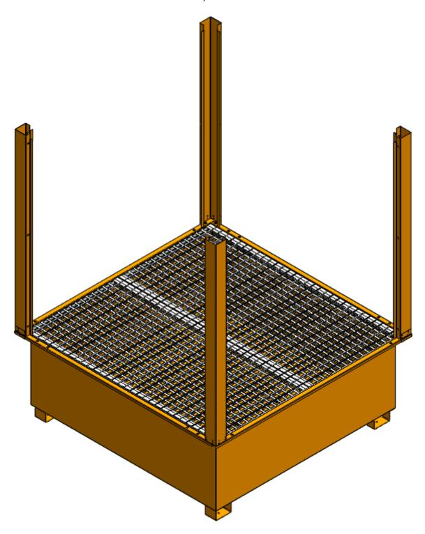
4. Position the short panel to the sump using M8 bolts, and secure it to the corner profile with M8 bolts and nuts.
